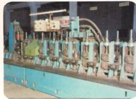
Tube Mill plant for high precision OD Tubes upto 2.0".
