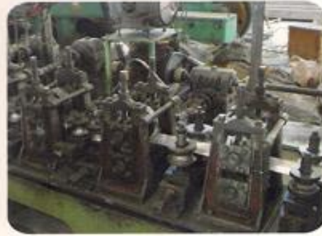
Tube Mill plant for 1/4" - 1" NPS and OD upto 1.50".
