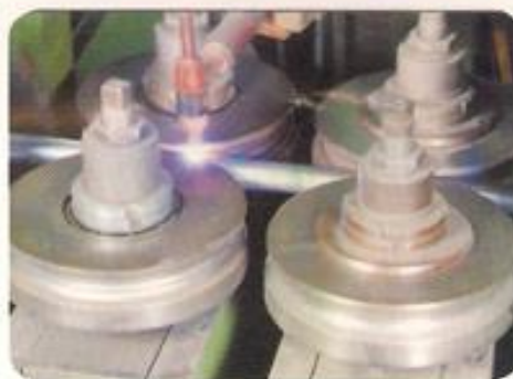
Tube Mill plant for high precision OD Tubes upto 2.0".
