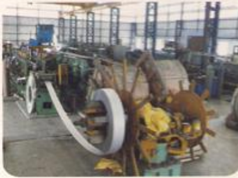
Tube Mill plant for 1.25" - 4" NPS and OD upto 4.0".
